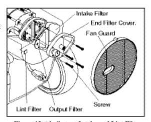
Figure 13. Air Output, Intake, and Lint Filters
